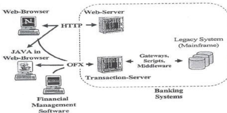
Figure 6.4. Scenario of a flexible Internet banking infrastructure integrating Web Information Systems, consumer client software, transaction services, and core banking systems.
